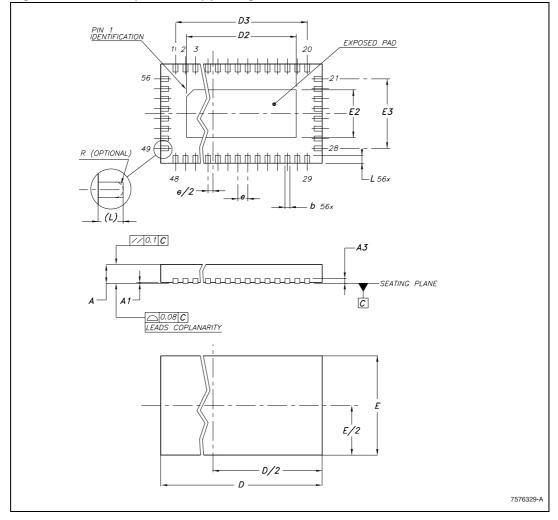
Figure 5. QFN56 (11 x 5 mm) package outline
